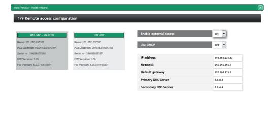
Select DHCP ON when the network settings are provided automatically by a DHCP server. In other case, select OFF and enter the network parameters manually (IP address, Netmask, Default gateway, Primary DNS Server, Secondary DNS Server). Consult network manager to get those parameters.
