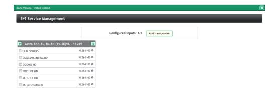
Repeat the same process with all the satellite transponders. In this example, the headend is formed by 2 HTL-STC modules, therefore you can receive up to 4 satellite transponders.
