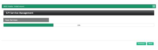
The headend will scan the input signal automatically. A progress bar will be displayed, indicating the percentage of the scanning that has been performed. When the scanning finish, the information of the detected multiplexes will be displayed. Select the desired services clicking in the check box next to those services. If you want to select all the services of a multiplex, push button.
